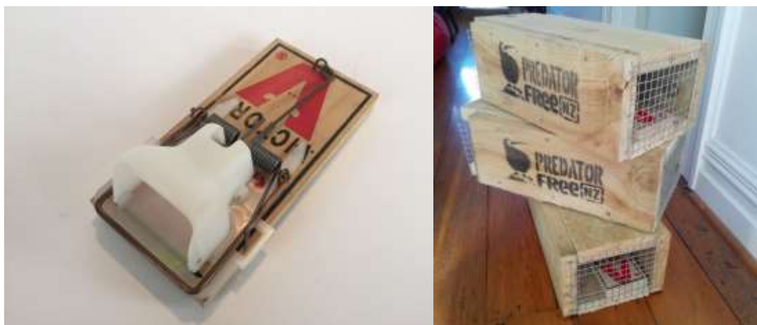
Figure 25: A standard 'Victor' rat trap with a shroud to encourage animals to enter the trap head on, an addition to increase the likelihood of clean kills, particularly for mustelids (left) and a fully set up Victor trap in a box to keep cats and birds safe, as well as to attempt to encourage animals to approach the traps head on.
